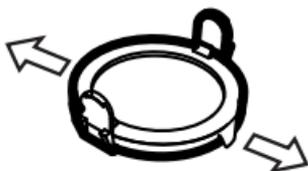
Pull out the clips located under the capsule
