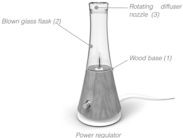
Carefully insert the glass flask (No.2) into the wooden base. Then insert the stopper (no.3) into the glass flask. Finally, connect the adapter to the mains socket (220-240V). **WARNING:** before inserting or removing the glass flask (no.2) make sure you have removed the rotatable nozzle (no.3) to avoid any risk of breaking. The blown glass parts are very fragile.
